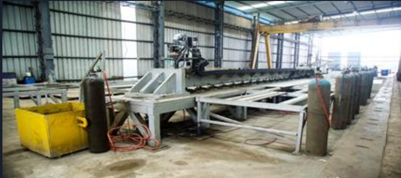
Clad Sheet Automatic Welding
